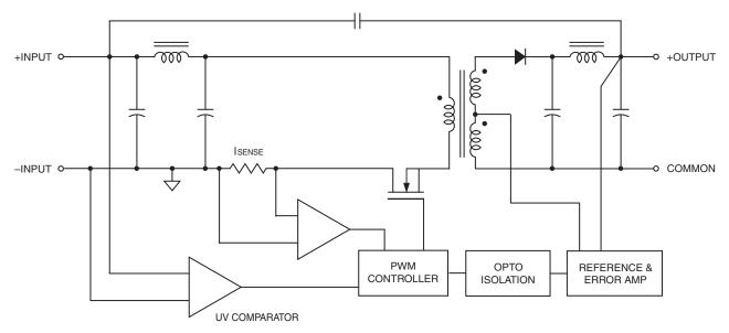
Figure 1. Simplified Schematic
