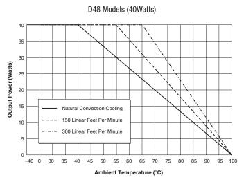
Figure 5a. Temperature Derating Without Heat Sink
