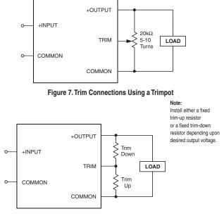
Figure 8. Trim Connections Using Fixed Resistors
