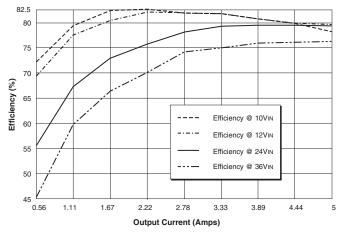
Figure 2c. Efficiency vs. Output Current and Input Voltage
