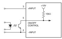
Figure 6. Driving the On/Off Control Pin
