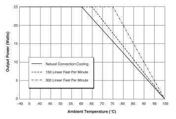
Figure 2b. Temperature Derating With Heat Sink
