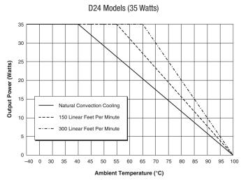
Figure 4a. Temperature Derating Without Heat Sink
