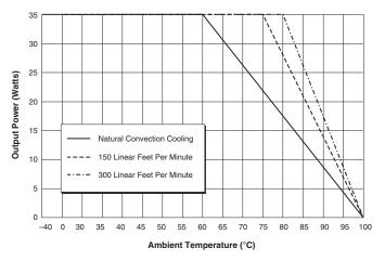
Figure 4b. Temperature Derating With Heat Sink
