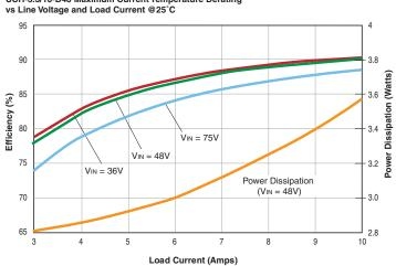
Isolated, "Half-Brick" 1.8–15V Output DC/DC Converters
