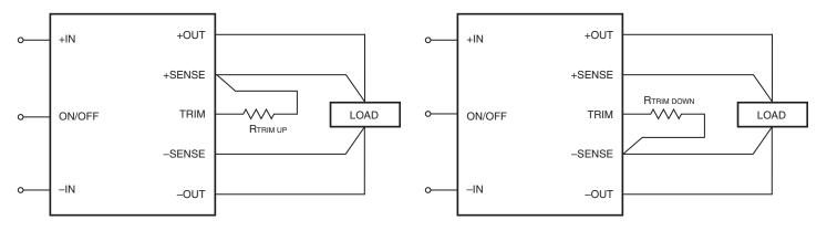
Figure 6. Trim Connections to Increase Output Voltages
