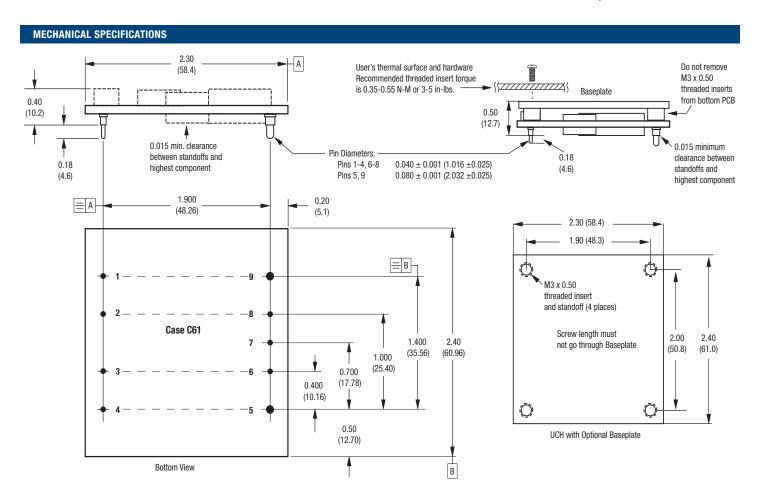
Standard pin length is shown. Please refer to the Part Number Structure for special order pin lengths.
