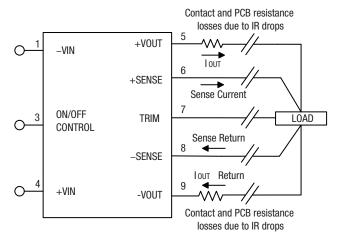
Figure 4. Remote Sense Circuit Configuration
