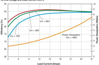
UCH-3.3/10-D24 Efficiency and Power Dissipation vs Line Voltage and Load Current @25°C
