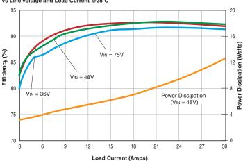
UCH-12/4.2-D48 Efficiency and Power Dissipation vs Line Voltage and Load Current @25°C
