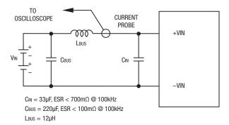
Figure 2. Measuring Input Ripple Current
