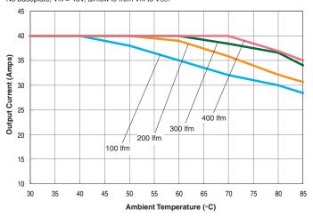
UCH-2.5/40-D48 Maximum Current Temperature Derating (at sea level) No baseplate, VIN = 48V, transverse airflow
