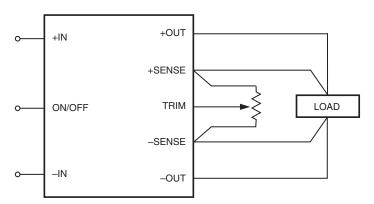
Figure 5. Trim Connections Using A Trimpot
