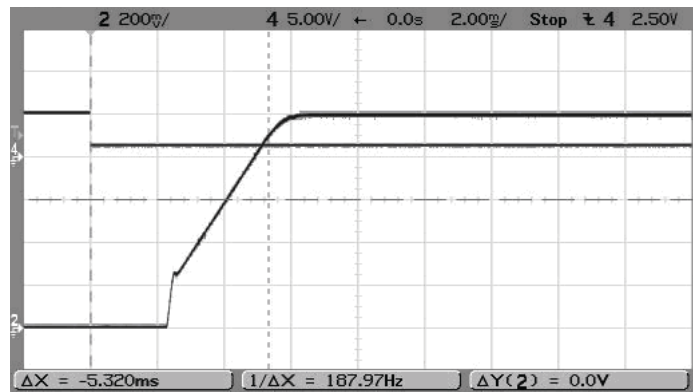
On/Off Enable Startup (V in =5V, V out =1.0V, I out =6A, Cload=0) Trace 4=Enable, Trace 2=Vout
