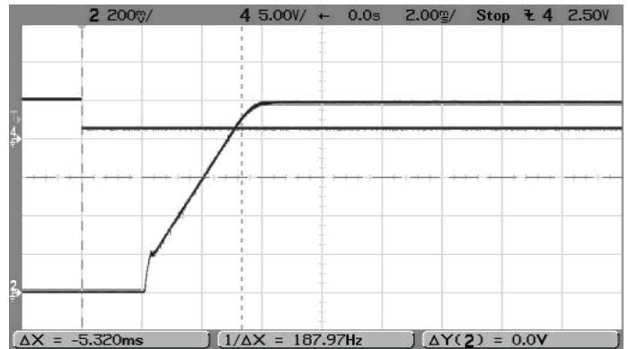
Step Load Transient Response (Vin=5V, Vout=1.0V, Cload=0, Iout=3A to 1.5A) Trace 2=Vout, 100 mV/div. Trace 4=Iout, 2.5A/div.
