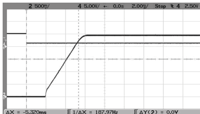
Step Load Transient Response (Vin=5V, Vout=2.5V, Cload=0, Iout=3A to 1.5A) Trace 2=Vout, 100 mV/div. Trace 4=Iout, 2.5A/div.
