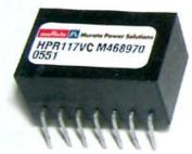
The HPR1XXVC Series uses advanced circuit design and packaging technology to deliver superior reliability and performance. A 170kHz push-pull oscillator is used in the input stage. Beatfrequency oscillation problems are reduced when using the HPR1XXVC Series with high frequency isolation amplifiers.
