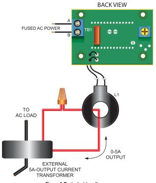
Figure 2. Typical wiring diagram
