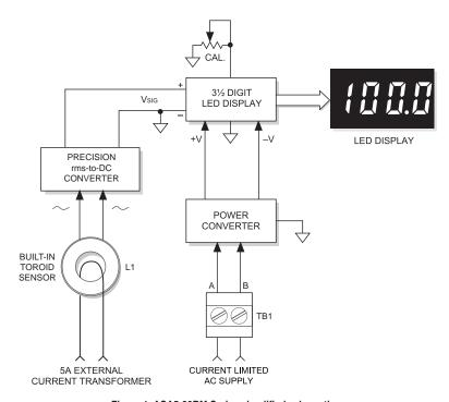
Figure 1. ACA5-20RM Series simplified schematic
